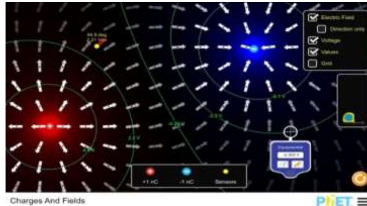
Figure 2.2: Visualization of "Invisible" Phenomena in PhET (Electric Field Lines)
